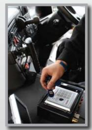
The first problem is when the driver releases the hand brake and attempts to drive away but can't because one of the vehicle interlocks (i.e. guard bar) is still active. If the driver leaves the cab at this point to clear the active interlock without re applying the hand brake first, the unattended vehicle, if parked on an incline, has the potential to roll away as soon as the interlock is reset.
